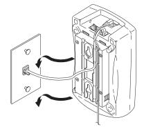
Plug the AC Adapter into a standard 120V AC wall outlet.
